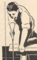
Proper position for cross-cutting
